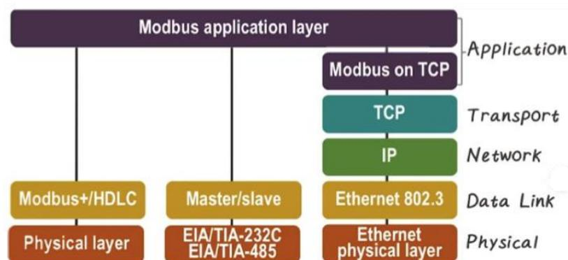
**Figure 4.** Industrial Layers (Pricop et al., 2017).
